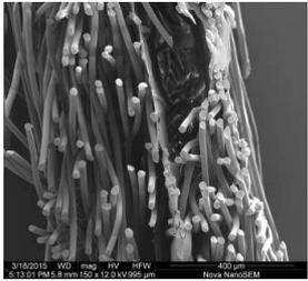
Innovative textile material that prevents penetration of dust mites and their allergens through the material based on mechanical collecting principle. The material also prevents migration of bed bugs and other parasites into the mattress and bedding.
