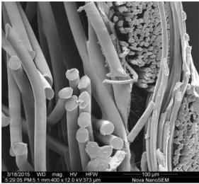
Anti permeability of AntiAllergy fabrics for dustmites, alergens and bed bugs is ensured by nanofibrous layer which is closed inside the textile membrane. Technically, the fabrics AntiAllergy are threelayred sandwiches with middle layer of nanofibrestructure. Mutual cohesion of single layers is secured by laminationtechnology.
